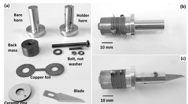
Figure 5. Parts of Langevin type ultrasonic device before assembling (a), K-6 lead-free BLT (b), prototype ultrasonic cutting device including lead-free KNN-KCN-ZnSn piezoceramics (c)
